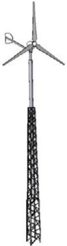
12 m lattice mast 1 x 3 m + 1 x 6 m lattice + 3 m pipe
