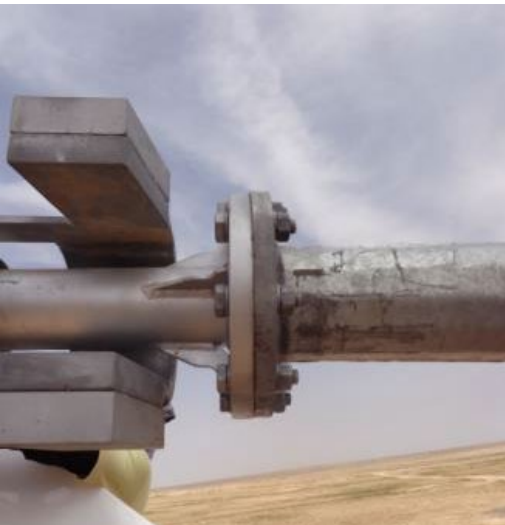
Picture 4: Machine gondola bolted to the mast while on the ground
