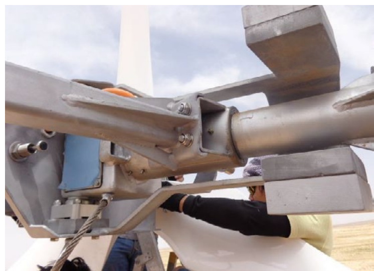
Picture 5: Pipe to the wind vane screwed to machine support. The 4 screws M12 are tightened with 50 Nm.
